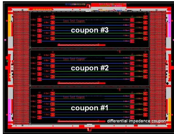
Figure 3 Location of Differential Impedance Coupon
