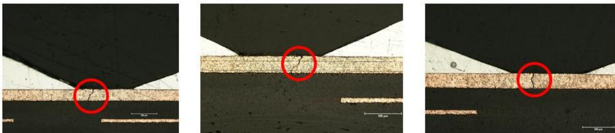
**Figure 10 – Examples of drop test failure mode “trace breakage” between SMDs**
