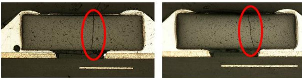
**Figure 11 – Drop test failure mode “component crack”**
