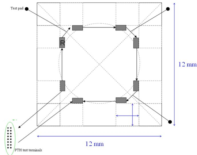
Figure 2 – Daisy chain test pattern on REL2000ec
