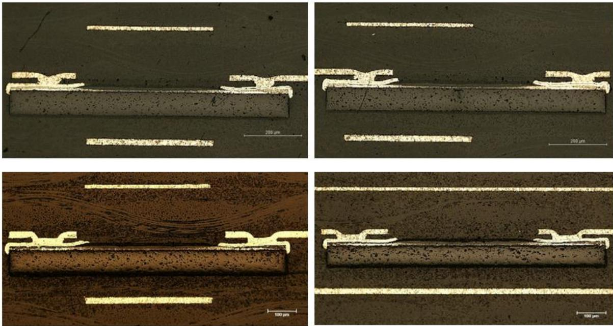
**Figure 12 – Examples of cross sections made from registered EC failure at 832 drops: no defect evident at component or interconnect**
