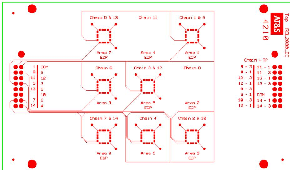
**Figure 3 – Outer layer circuit pattern of REL2000ec**
