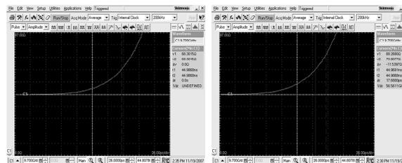
**Figure 10. Electrical Length Before Heat Exposure and Electrical Length After Heat Exposure (17.68 psec shorter)**
