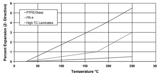
**Figure 6. Expansion as a Function of Temperature**
