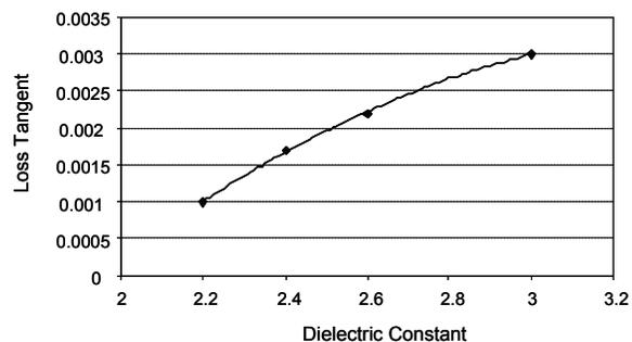
Figure 2. Loss Tangent vs. Dielectric Constant for PTFE/Glass Laminates at 10 GHz
