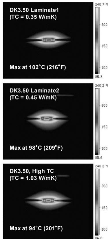
**Figure 5. Thermal Images of Heat Dissipation around RF Power Resistors and Max Temperature Reduction due to Higher Thermal Conductivity at 3.5 DK**
