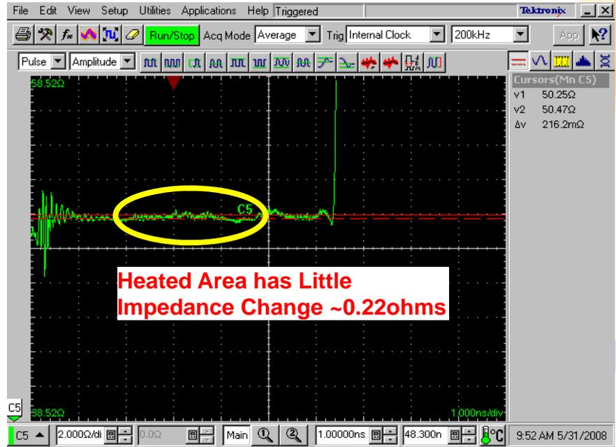
Temperature Effects on Impedance of **High TC** DK3.5 Laminate (**-9 ppm/° C**) **at 125° C**
