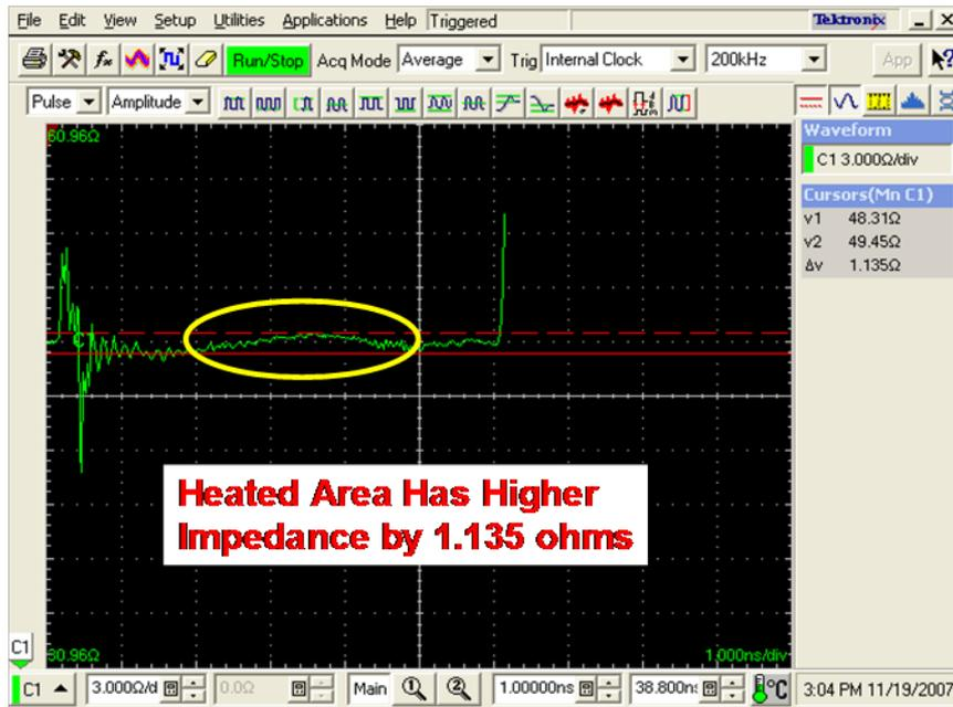
Temperature Effects on Impedance of a Standard **-150 ppm/° C** DK3.5 Material **at 125° C**
