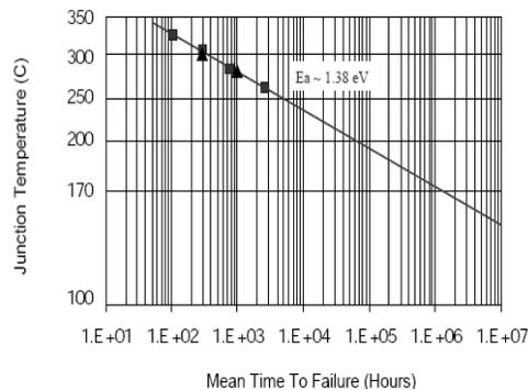
**Figure 1 Arrhenius Chart Junction Temperature Failure Rate**
