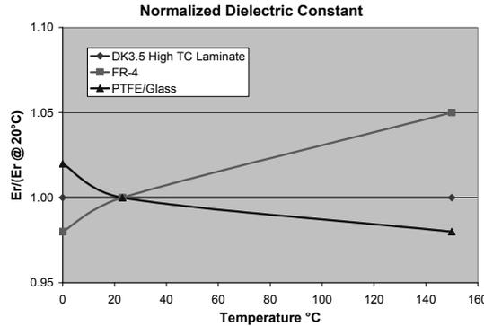
Figure 7. Change in Dielectric Constant over Temperature
