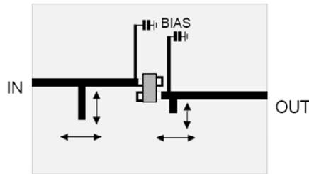
**Figure 8. Power Amplifier Impedance Matching Networks**
