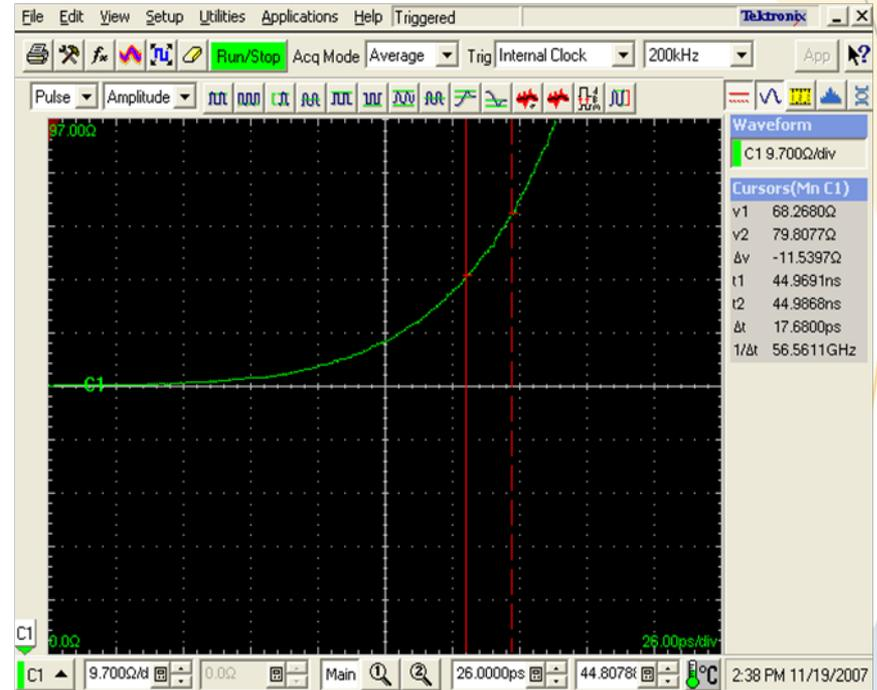
**Electrical Length Before Heat Exposure and Electrical Length After Heat Exposure at 125° C (with 17.68 psec shorter in 5.80 nsec microstrip line on the Standard laminate)**
