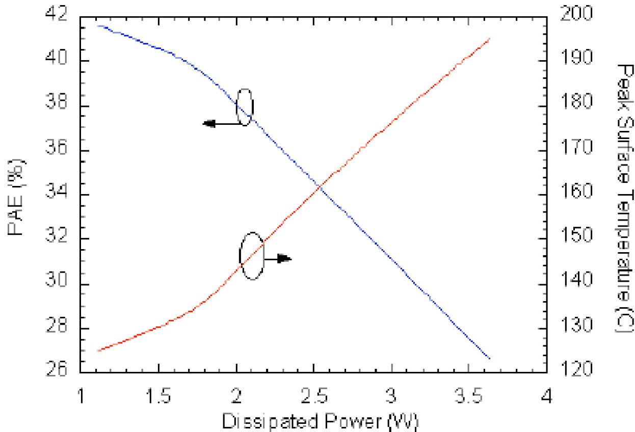
S. Nuttinck, R. Mukhopadhyay, C. Loper, S. Singhal, M. Harris, J. Laskar, "Direct On-Wafer Non-Invasive Thermal Monitoring of AlGaIn/GaN Power HFETs Under Microwave Large Signal Conditions."
