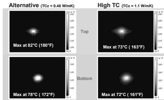
**Figure 4. Thermal Images of Heat Dissipation around RF Power FET Transistors and Associated Max Temperature Reduction due to Higher Thermal Conductivity**
