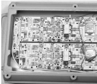
**Figure 3. A Microwave Power Amplifier Board**
