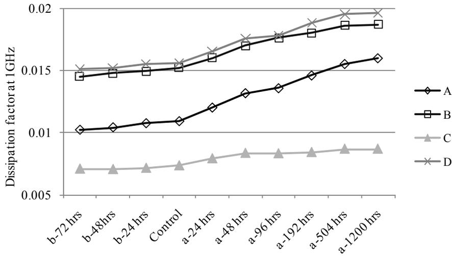
**Figure 9 Dissipation factor values in different moisture test conditions**
