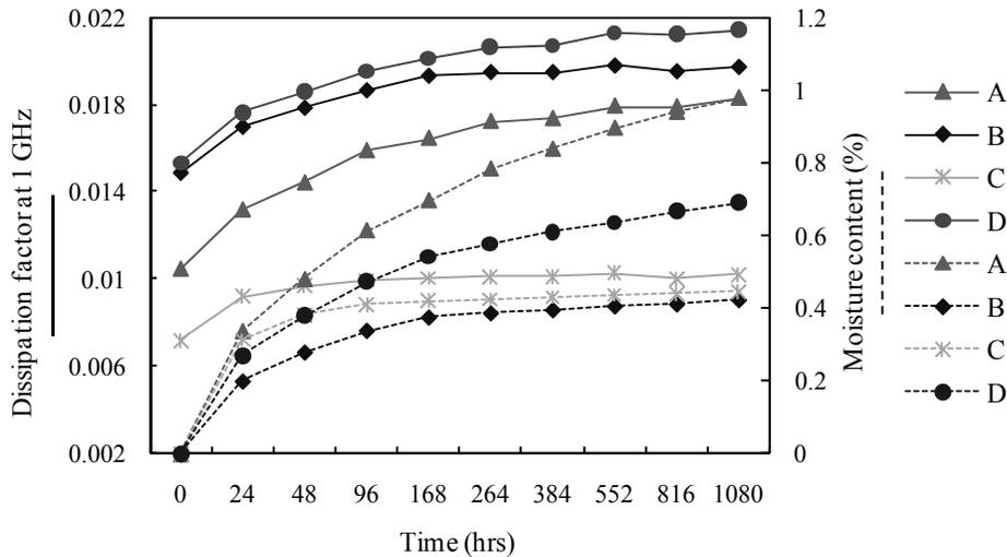
**Figure 5 Dissipation factor at 1GHz and absorbed moisture content as a function of exposure time at 85°C/85% RH**
