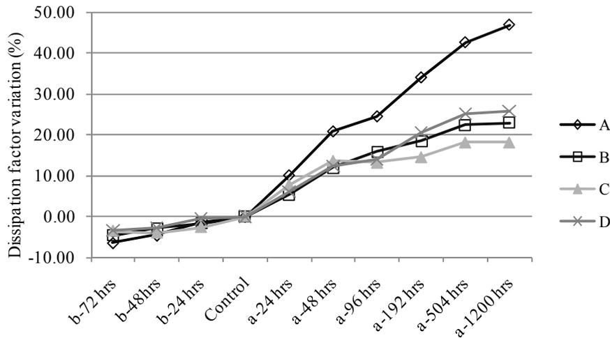
**Figure 11 Dissipation factor variation in different moisture test conditions**
