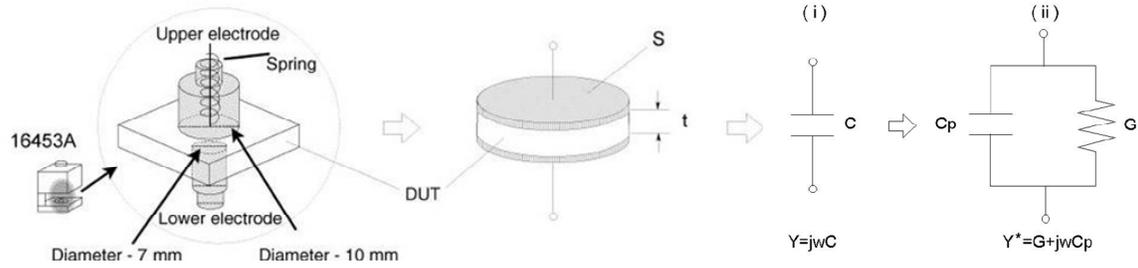
**Figure 1 Schematic of capacitor method used in 16453A**
