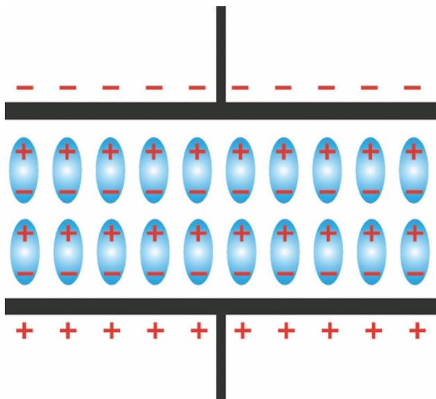
Schematic view of a capacitor
