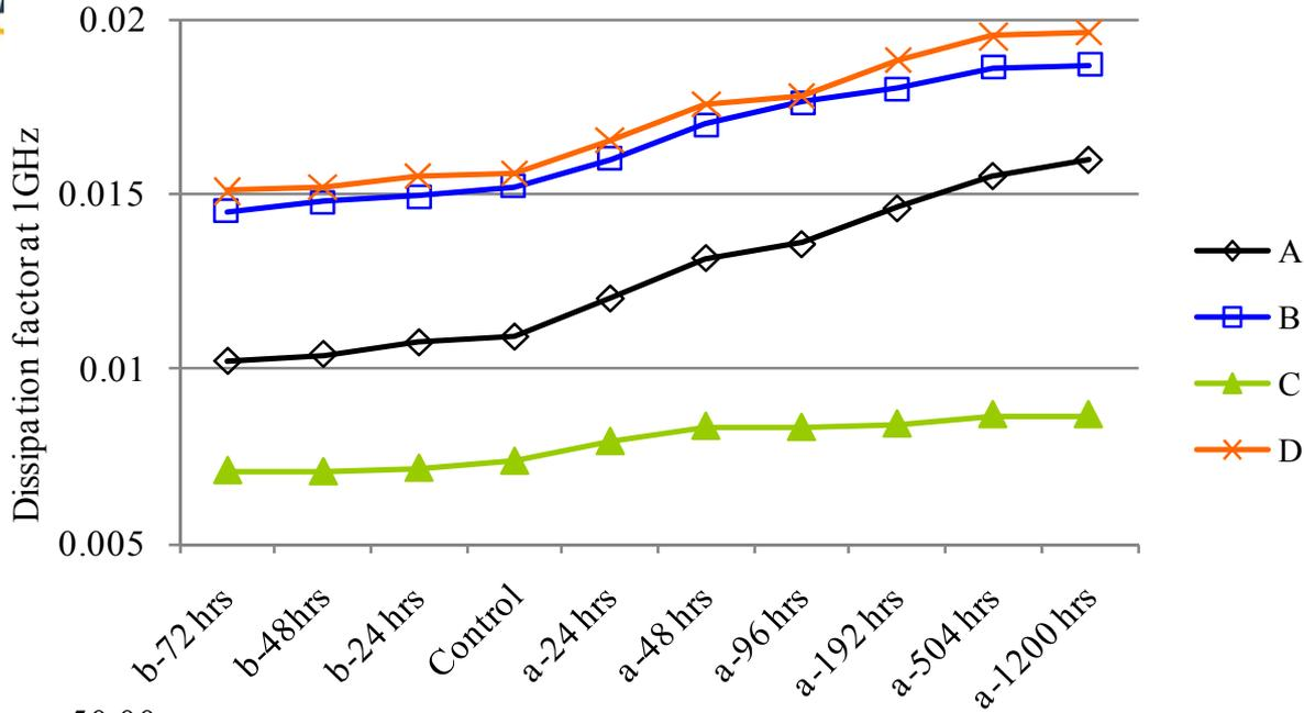
$D_f$  increased ~46.7% compared with the control set after preconditioned according to IPC test standard.
