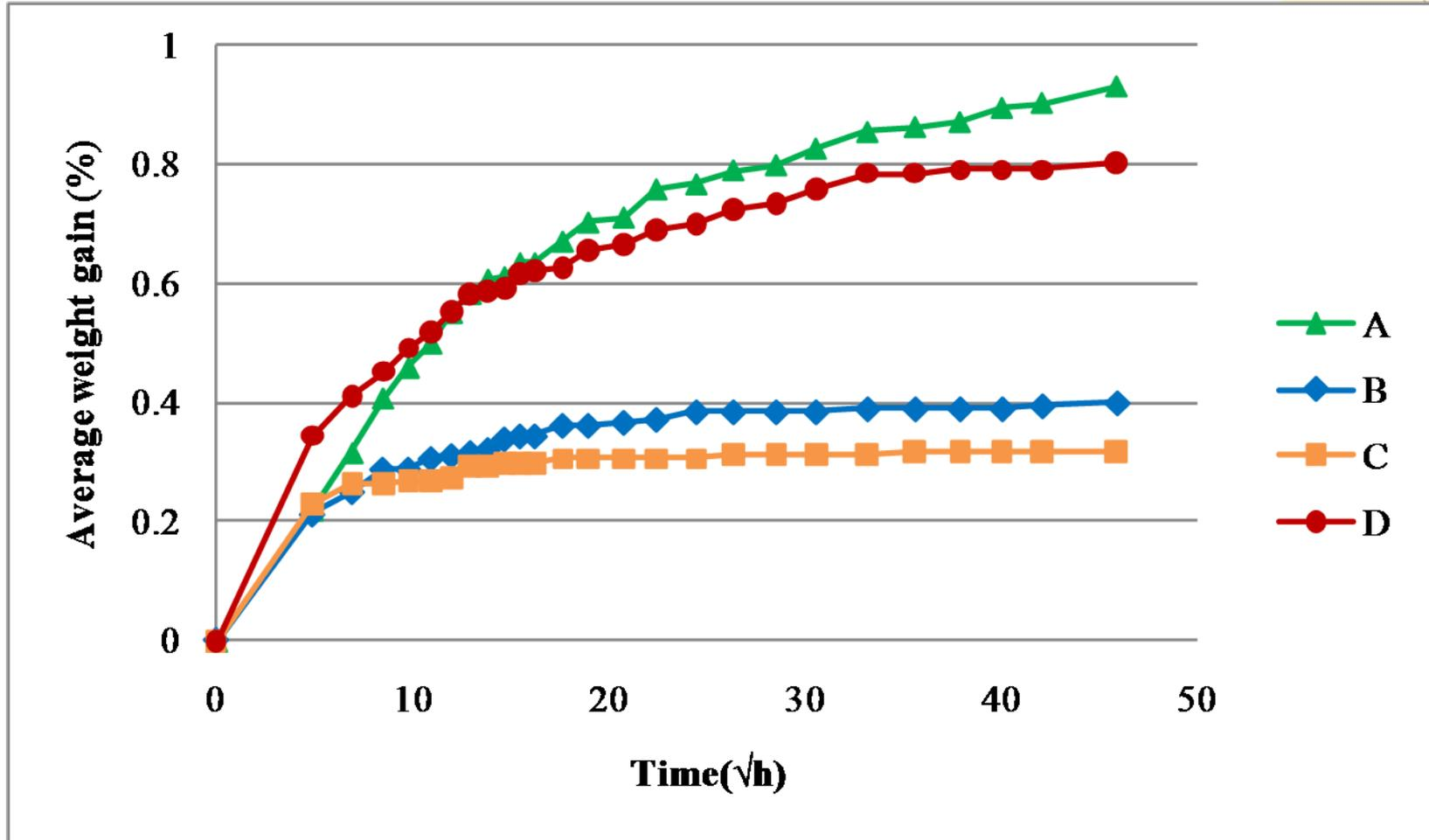
Moisture absorption experiments were conducted on two coupons (10mm × 10mm and 20mm × 20mm) of each PCB material which were exposed in 85°C and 85% RH condition and the coupons were taken out of chamber to measure weight at increasing time intervals.
