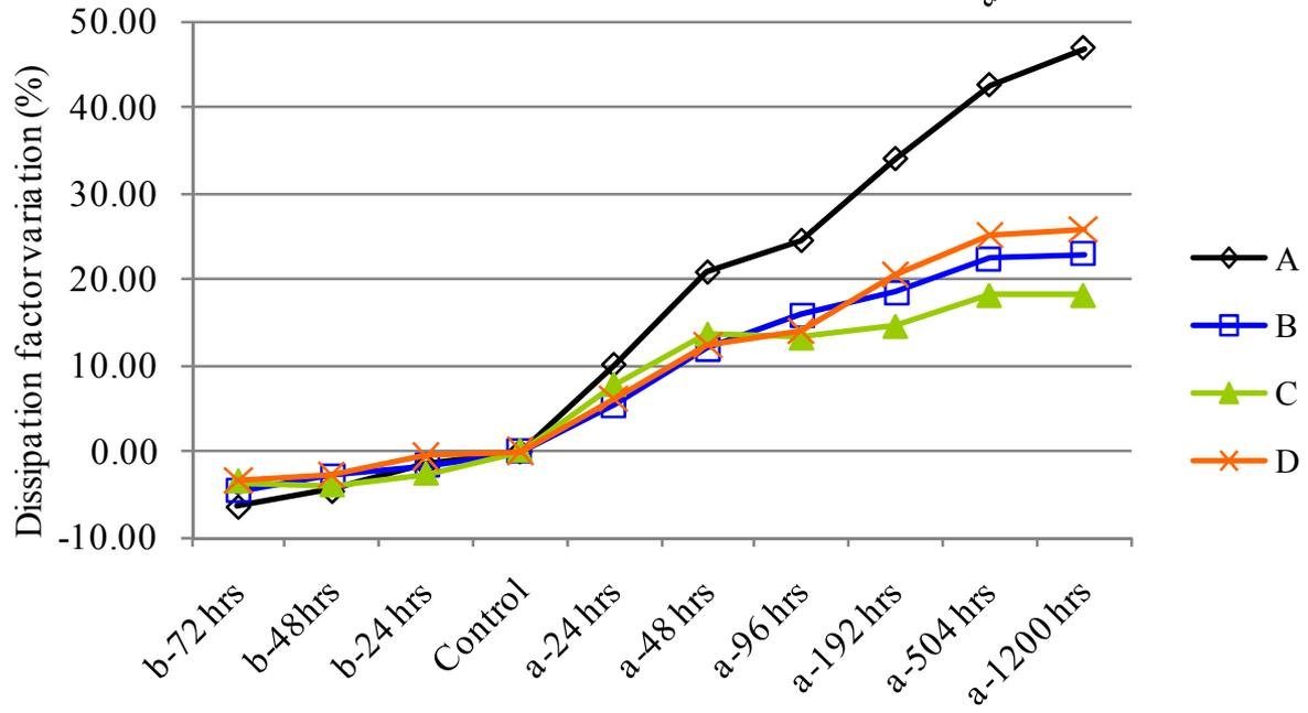
Preconditioning procedure outlined in IPC-TM-650 2.5.5.9 test standard can not account for different moisture content.
