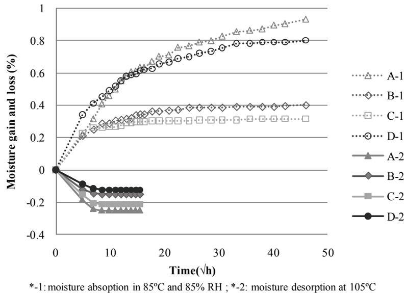
**Figure 2 Rate of moisture absorption and desorption for four materials (average values of two test coupons)**
