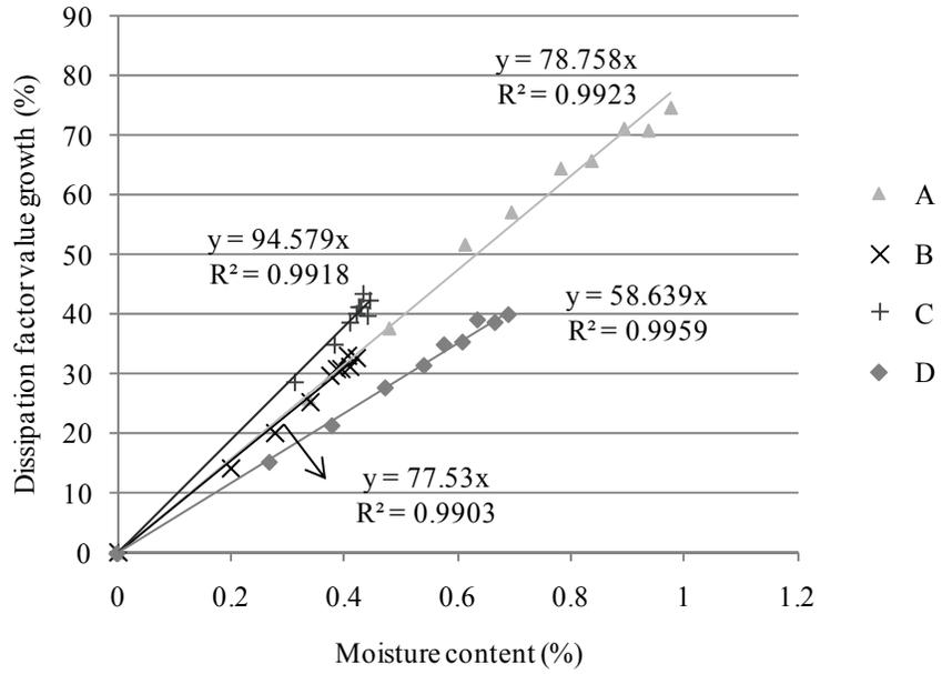
**Figure 7 Dissipation factor value changes with different moisture content**
