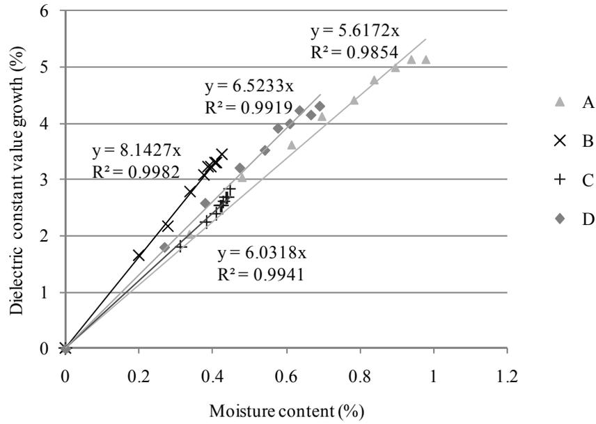
**Figure 6 Dielectric constant value changes with different moisture contents**
