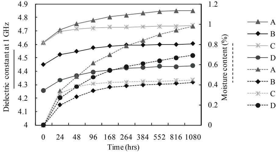
**Figure 4 Dielectric constant at 1GHz and absorbed moisture content as a function of exposure time at 85°C/85% RH**
