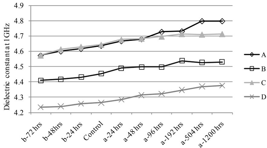
**Figure 8 Dielectric constant values in different moisture test conditions**
