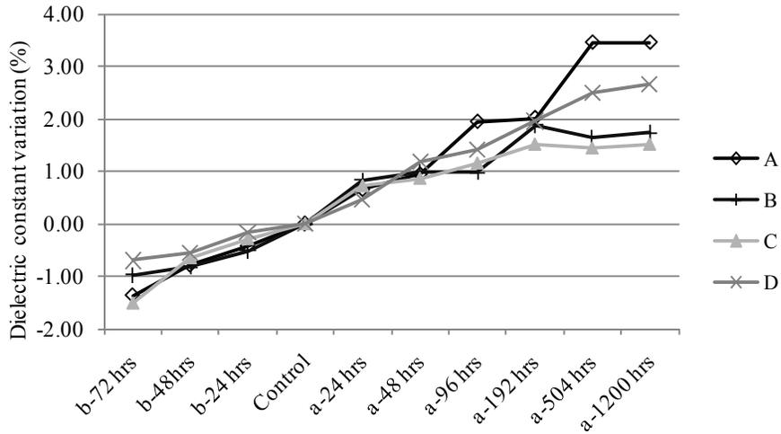
**Figure 10 Dielectric constant variation in different moisture test conditions**
