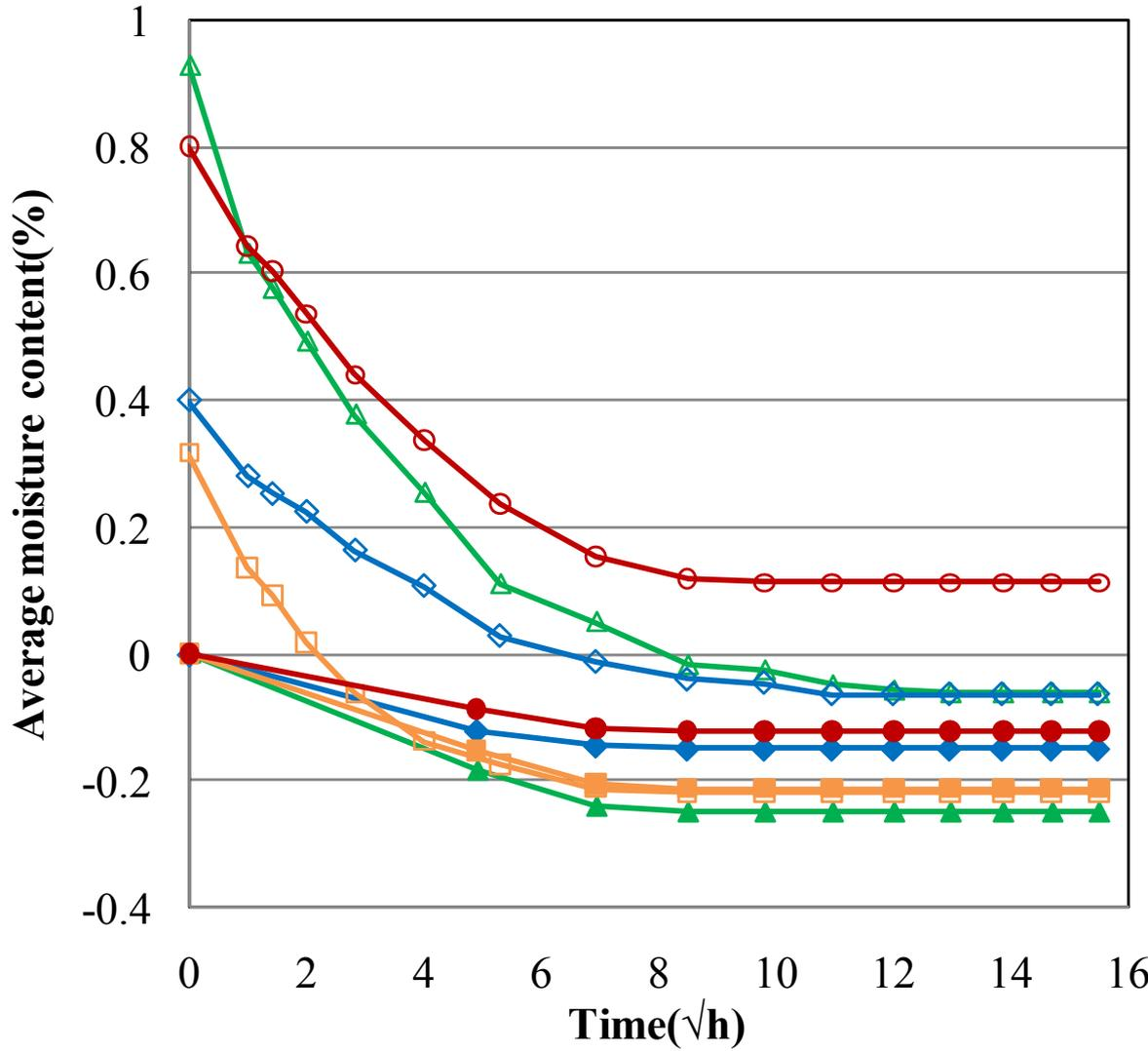
Moisture desorption experiments were baked at 105°C on two kinds of specimens:
