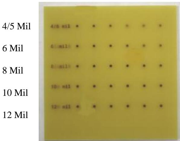
**Figure 1-Via Test Board**
