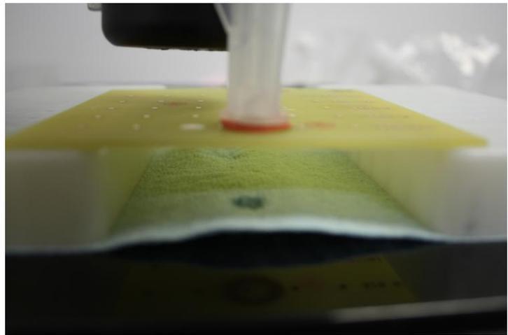
**Figure 2- Localized Extraction Example over 4/5 Mil via**
