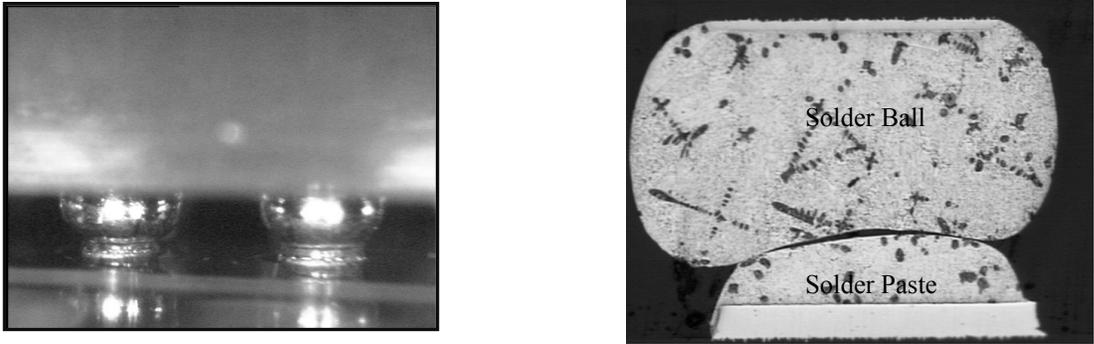
Figure 1: Sideview and Cross-Section Images of a Head in Pillow Defect
