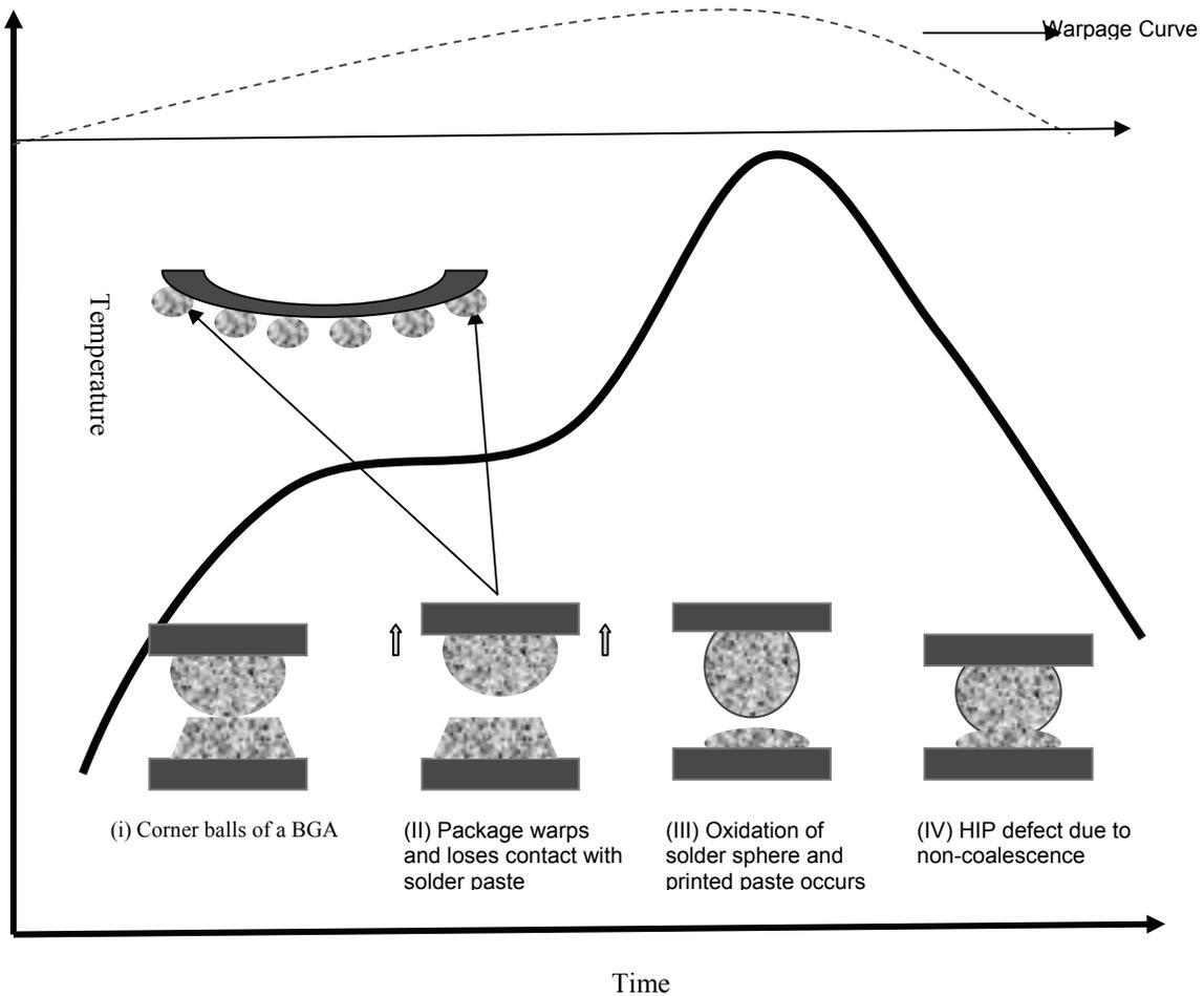
Figure 2: Mechanism of Head in Pillow Defect Formation
