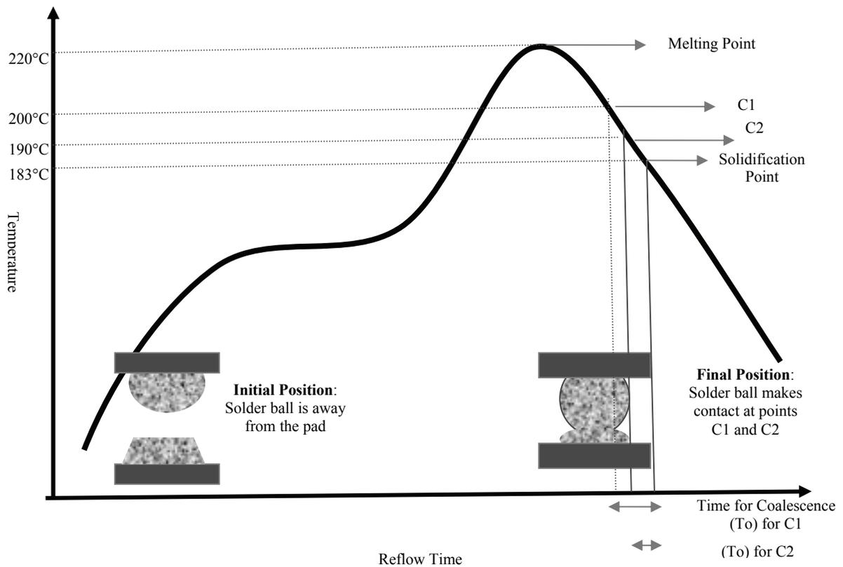
Figure 6: Conditions for HiP Defect
