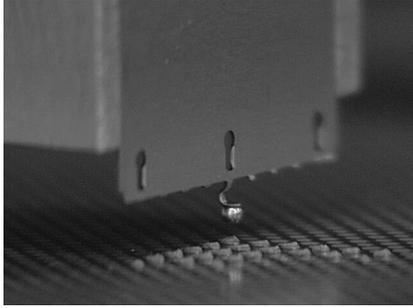
Figure 7: Solder ball position at preheat stage
