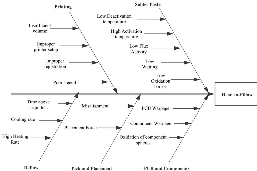
Figure 3: Fishbone diagram for HiP defect
