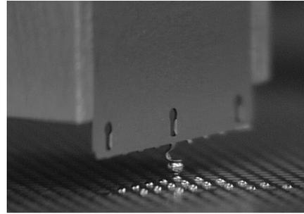
Solder ball during cool down stage making contact with solder paste.
