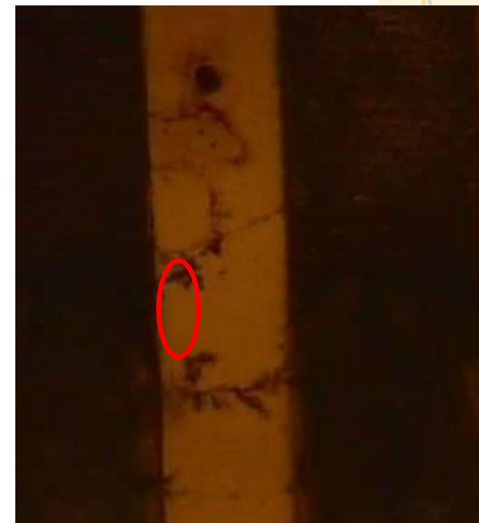
Dendrites on SIR coupon after processing with halide free flux
