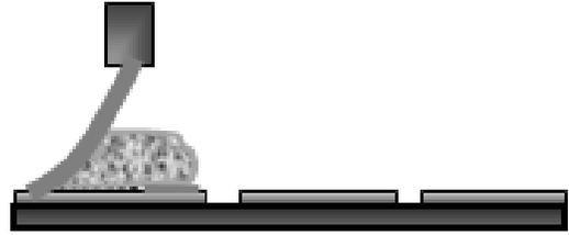
**Figure 3b.** Attack angle  $<60^{\circ}$  during print stroke
