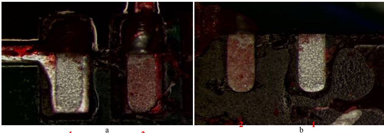
Figure 10: Dye and Pry results of a QFN-20 showing dye penetration through the bulk solder: a- board side; and b- component side
