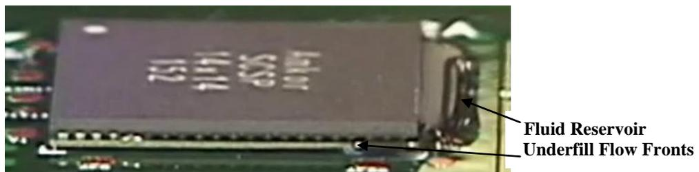
Figure 1: Underfill reservoir and Flow Fronts
