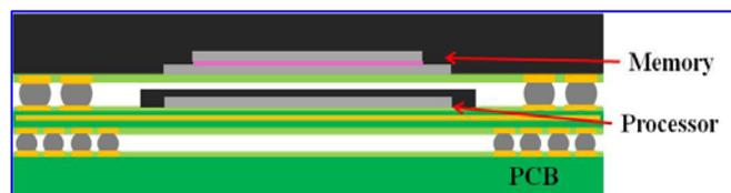
**Figure 1: Package on package technology**
