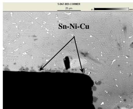
**Figure 11 - Cross section of a LF-BGA soldered with SnPb-paste; the sample was prepared with a reflow peak temperature of  $225^{\circ}\text{C}$  (secondary electron images).**
