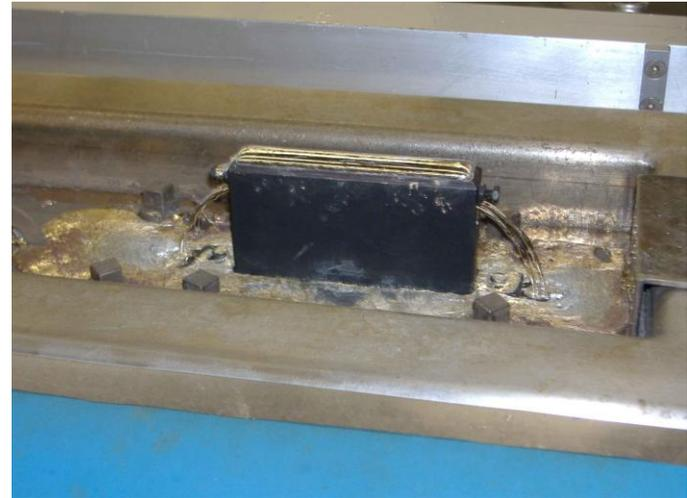
Process 2: The Premier Rework RW116 machine was used for initial component installation, component removal, and second component installation. This process used the hybrid nozzle design, to minimize solder flow at contact with rework coupon while maintaining adequate heat transfer.
