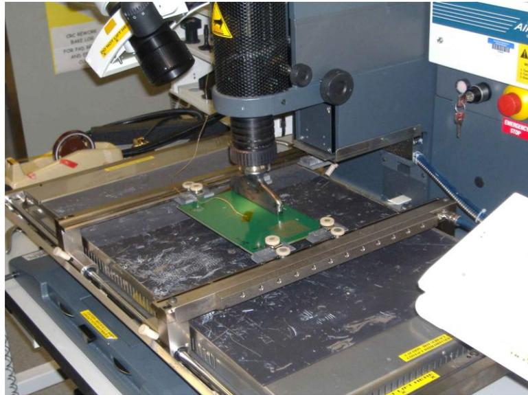
Process 3: The Premier Rework RW116 was used for the initial and second component installation. This process used the standard nozzle design for component installation. The Air Vac DRS25 was used for component removal.
