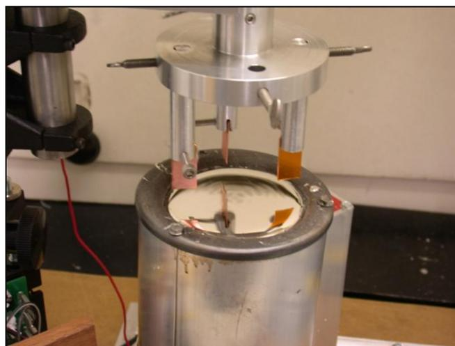
**Figure 3. Experimental setup of the dynamic copper dissolution experiments.**
