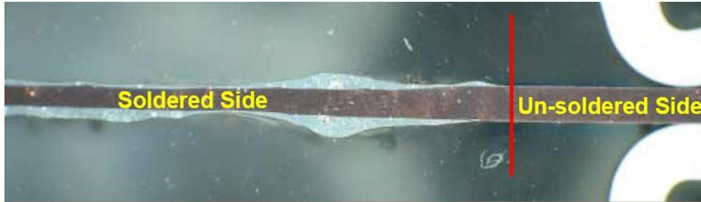
**Figure 4. Test coupon after copper dissolution test.**
