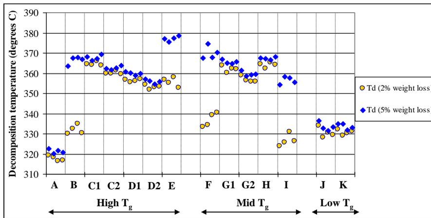
Figure 5: Effect of lead-free soldering exposures on T<sub>d</sub> (2% and 5% weight loss) of the laminates
