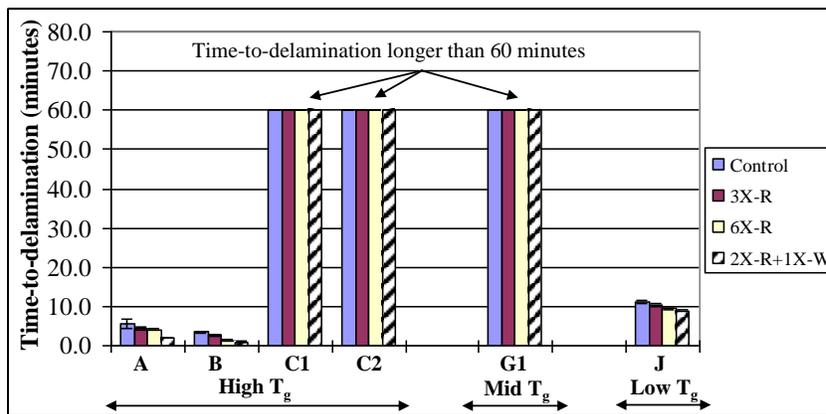
Figure 6: Effect of lead-free soldering exposures on T-260
