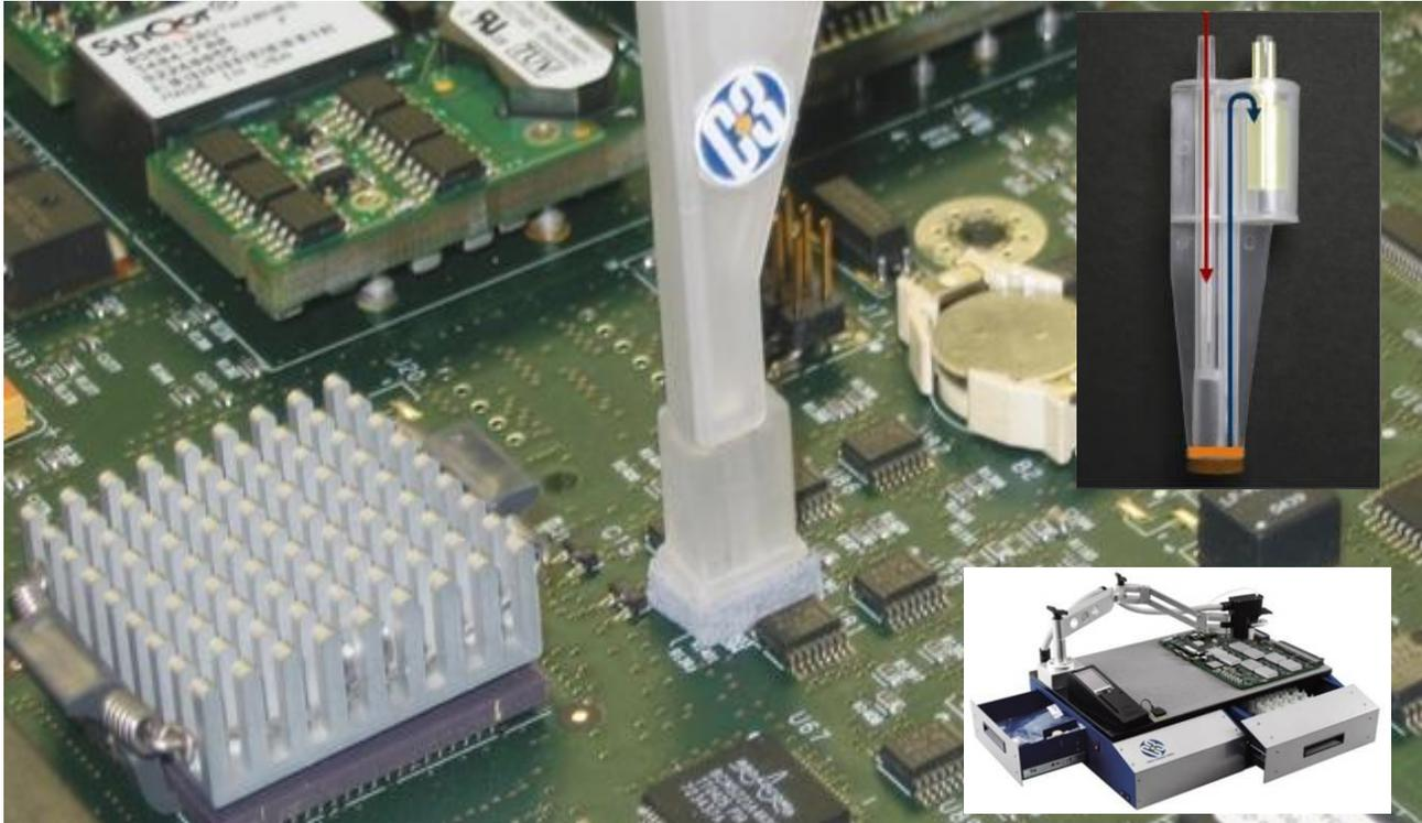
**Figure 11 –Cleanliness test system**
