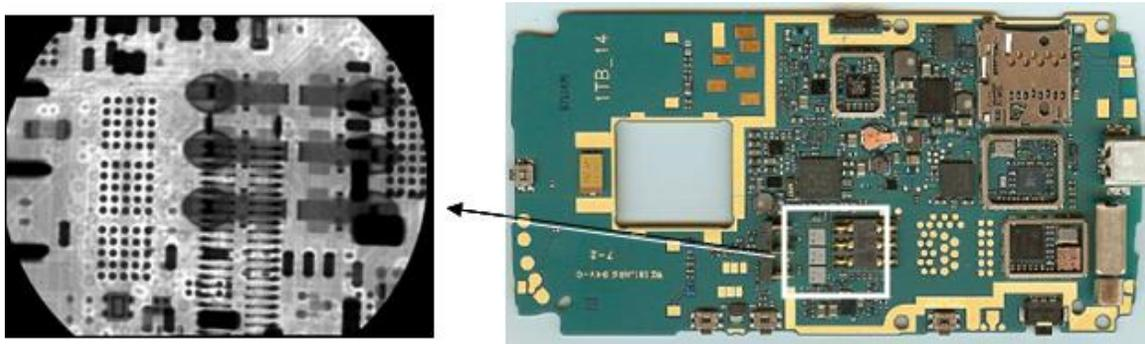
**Figure 1. Example of wireless handset with extensive use of wafer level BGA packaging.**
