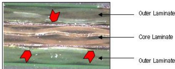
**Figure 2. Inner-layer separation within the PCB structure.** (source: Cookson)
