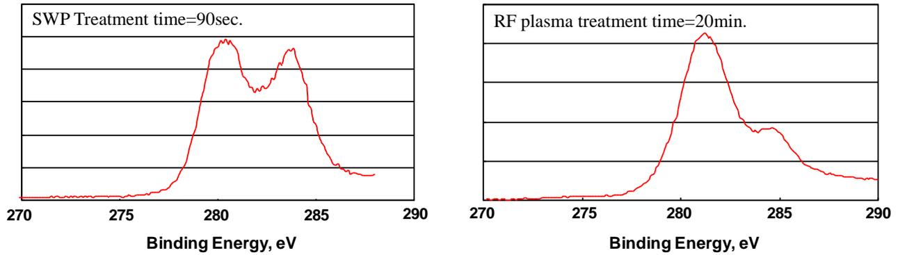
**Fig. 5. C1s XPS spectra after SWP and RF plasma treatment**
