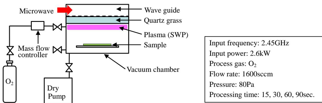
Fig. 1. Schematic diagram of microwave plasma (SWP)
