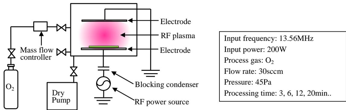
**Fig. 2. Schematic diagram of radio frequency (RF) plasma**
