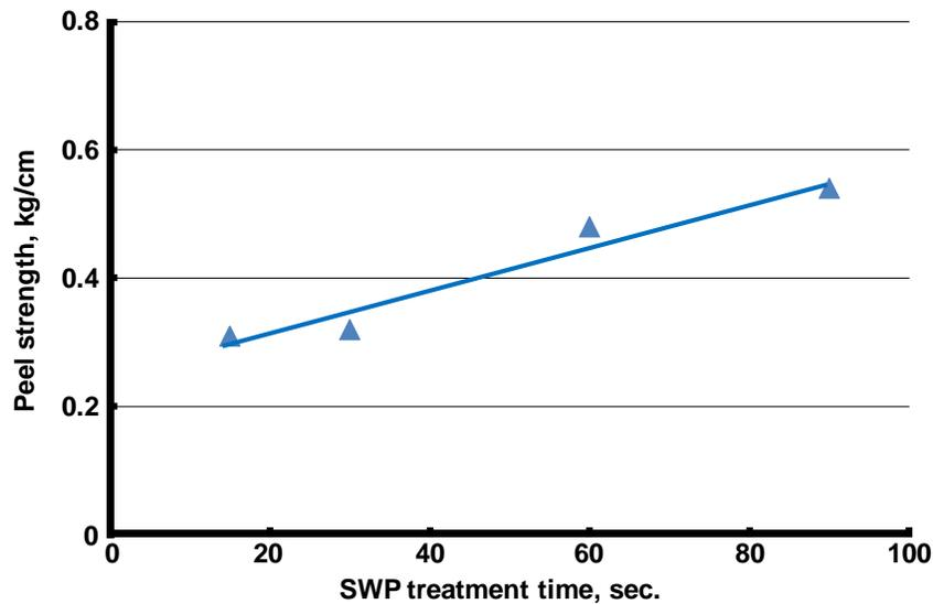
Fig. 7. Peel strength of electroless Cu plating with SWP treatment
