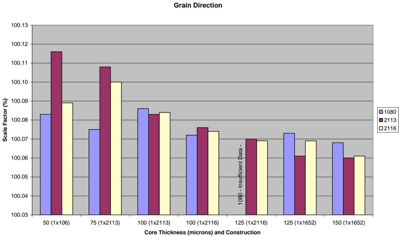
Figure 3 – Effect of Adjacent Prepreg on Average Required Scale Factor in the Grain Direction
