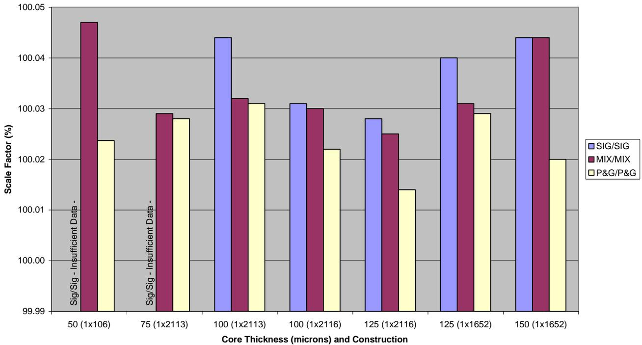
Figure 2 – Effect of Copper Distribution on Average Required Scale Factor in the Fill Direction
