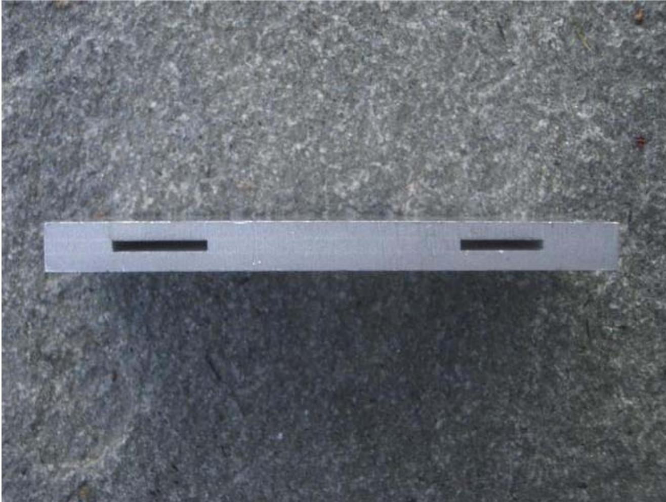
**Figure 7: Cooling Channels**
