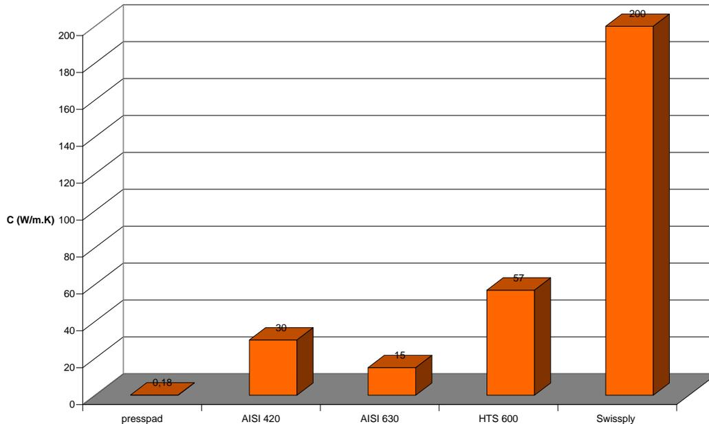
**Figure 2: Heat Conductivity**
