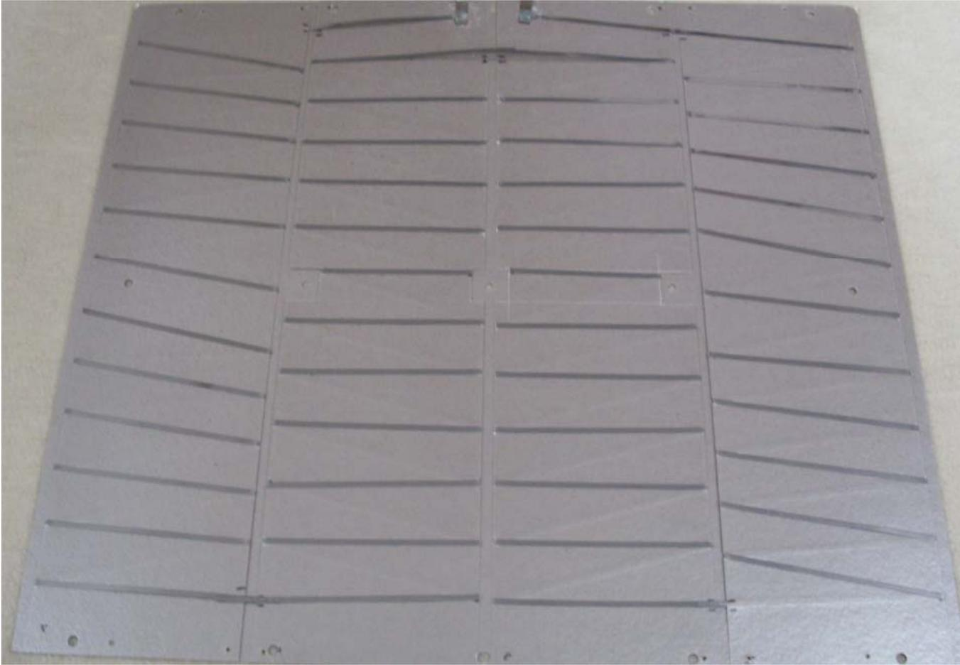
**Figure 5: Heating Element**
