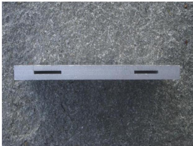
Figure 7: Cooling Channels
