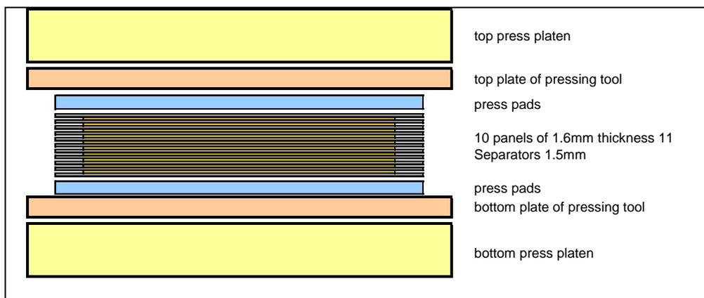
Figure 1: State of the Art Pressing Technology
