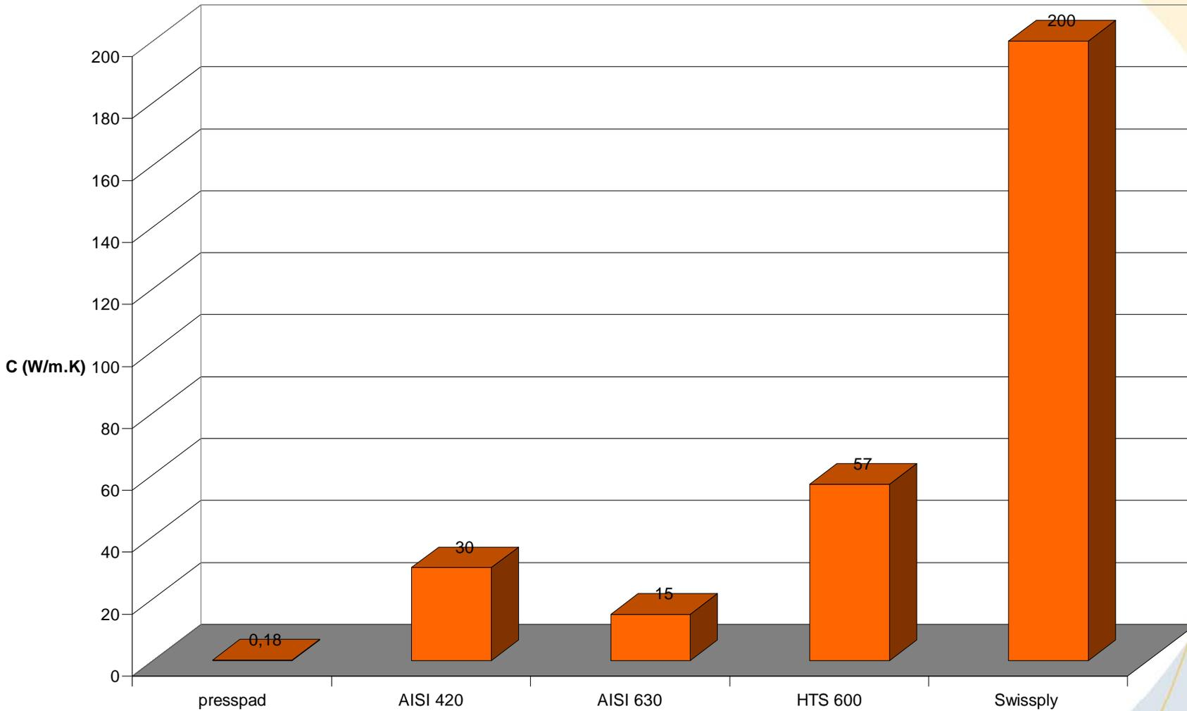
**Figure 2: Heat Conductivity**
