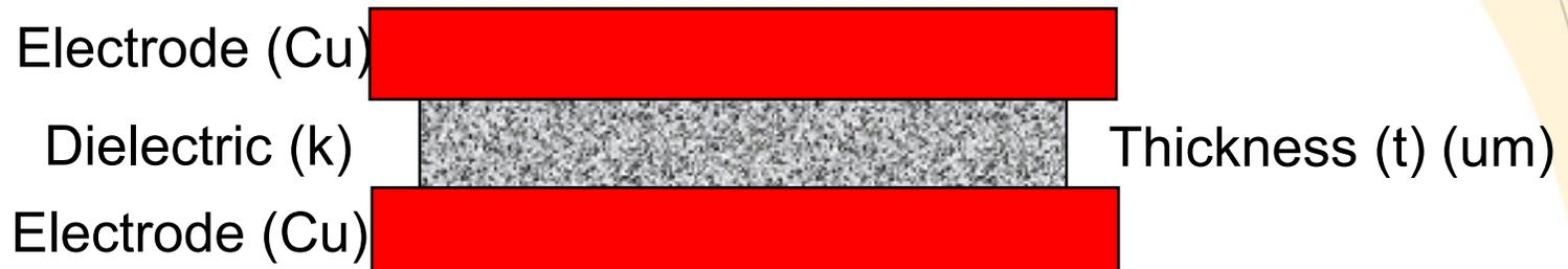
$$\text{Capacitance/Area} = 0.885 \text{ k/t (nF/cm}^2\text{)}$$
