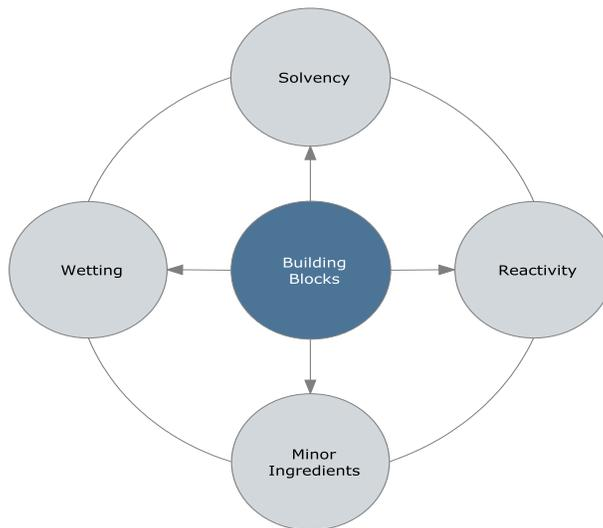
**Figure 3 Electronic Assembly Cleaning Material Building Blocks**
