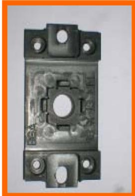
**Eliminated the Compression spring and o-ring by transferring the spring effect to the suction cup**
