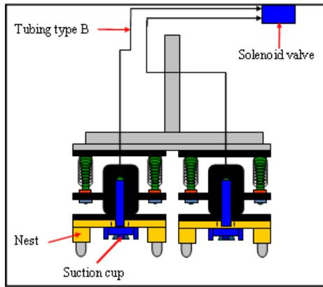
Figure 7: RFS Cone chuck after changes made
