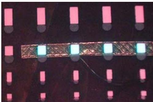
**Fig. 8 Flexible EL dot array made by screen-printing process**
