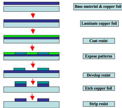
**Fig. 4 Basic patterning process of the copper foil circuits**
