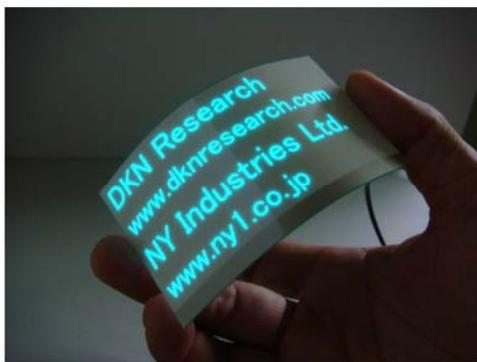
**Fig. 6 Example of the flexible EL made by all screen-printing process**
