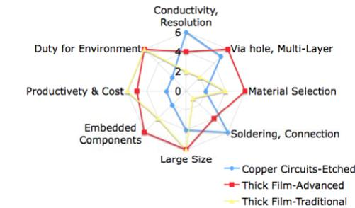
Fig. 1 Comparison of the circuit manufacturing processes
