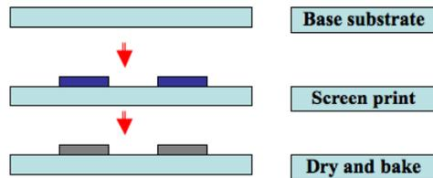
Fig. 3 Basic patterning process of the thick film circuits
