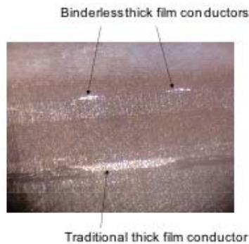
**Fig. 9 Cross Section Photo of the Thick Film Conductors**
