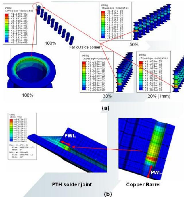
**Fig. 9 Inelastic strain concentration on the copper barrel for various hole fills (a) and zoomed view of 10% hole fill case (b) under thermal cycling (5mm PCB).**
