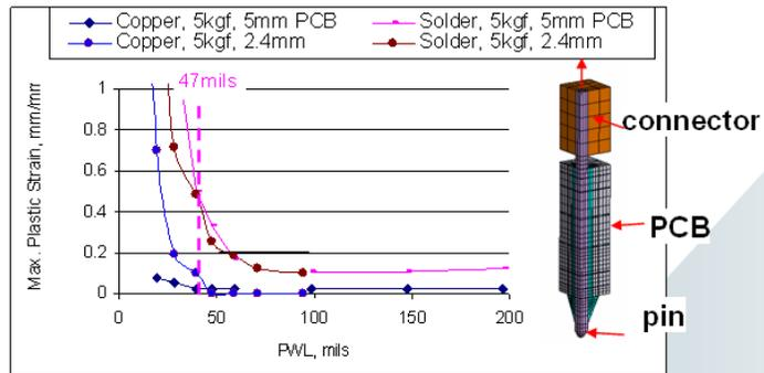
**Fig. 11 Plastic strain vs. PWL at various board thicknesses at a pull force of 5 kgf (1 kgf=2.247 lbf).**
