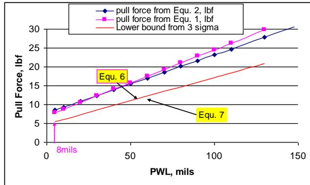
**Fig. 12 Impact of PWL on pull force from empirical calculation.**
