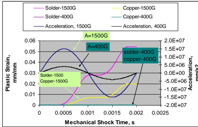
Fig. 14 Response of maximum plastic strain of PTH solder joints from mechanic shock (3.1 mm board).
