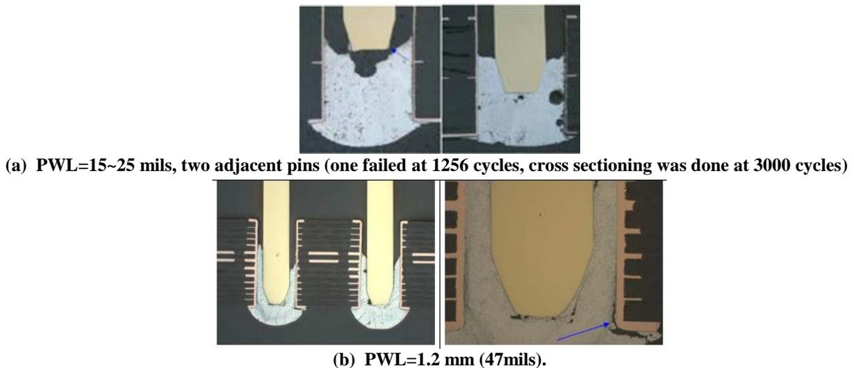
Fig. 8 PTH solder joint failures (a) and non failure (b). Note: board thickness=2.4 mm (94 mils) and no pin protrusion,
