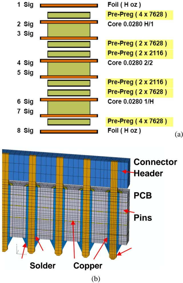
**Fig. 2 Layer structure in the test vehicle (a) and FEA (b).**
