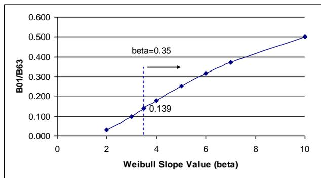
Fig. 4 B01/B63 vs. Weibull slope for PTH vias.
