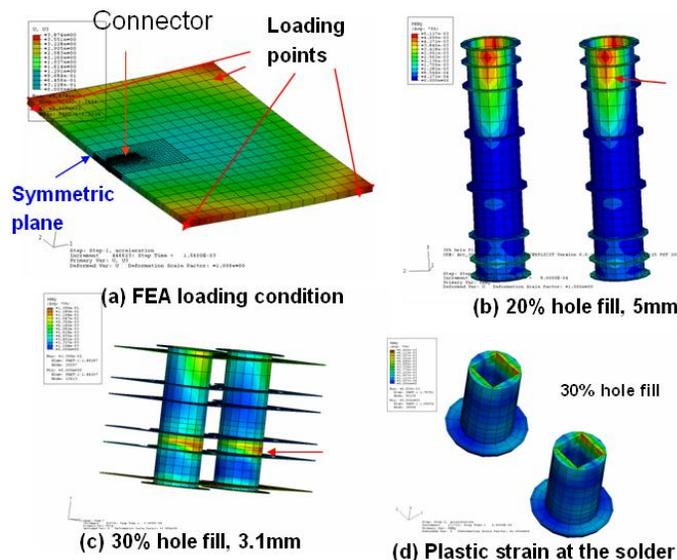
Fig. 13 FEA models for mechanical shock at 1500 G.
