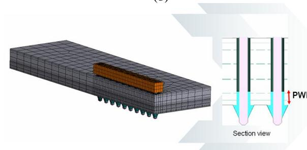
(c) **Fig. 1 (a) Test vehicle, (b) Cross sectioning view of PTH, and (c) FEA model including a connector**
