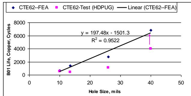
**Fig. 6 Hole size impact on the via reliability (B01 life, CTE at z-axis=62ppm/C, 3.1mm board).**
