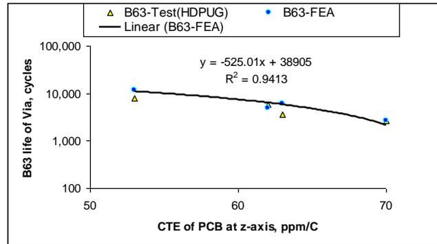
**Fig. 5 Characteristic life of PTH vias by FEA in comparison with the testing results (3.1 mm board).**
