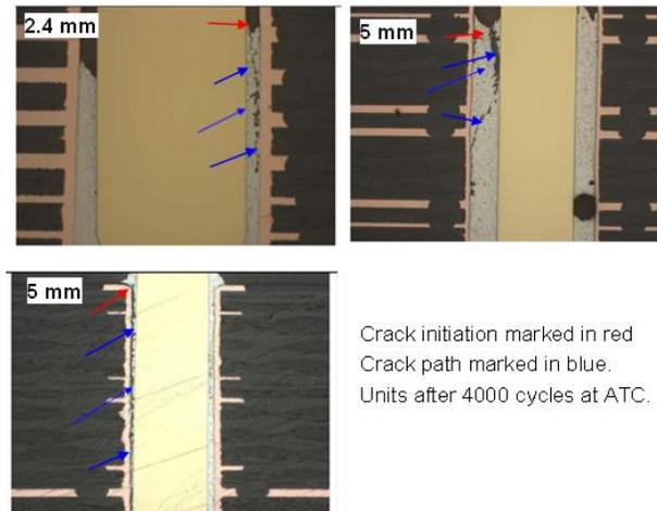
Fig. 7 Cracking of PTH solder joints after 4000 ATC cycles.
