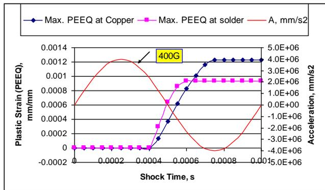
Fig. 15 Response of maximum plastic strain of PTH solder joints from mechanic shock at 400 G (2.4 mm board).
