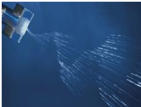
Figure 3 – Oscillating nozzle spray pattern.
