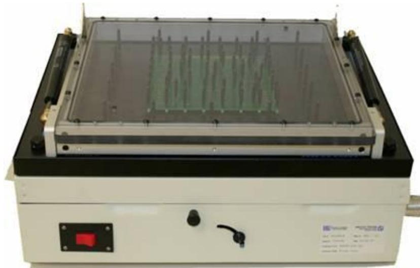
**Figure 1. Pin-Testability Fixture**
