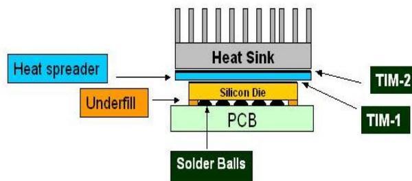
Fig. 1. Example of TIM 1 and 2 in Flip Chip Package
