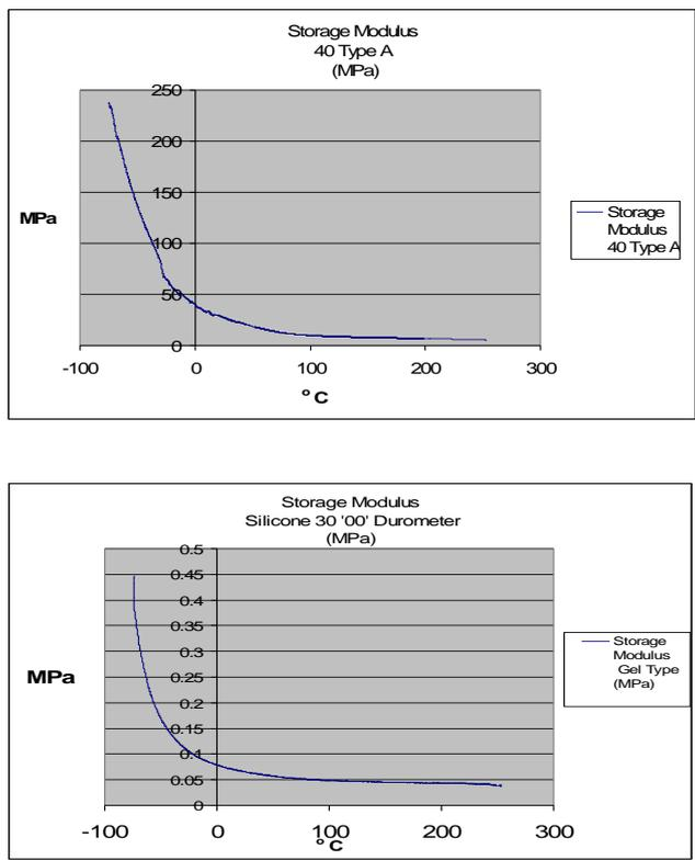
**Fig. 3. Average Elastic Modulus (MPa) versus Temperature of Silicone 1 and 2**
