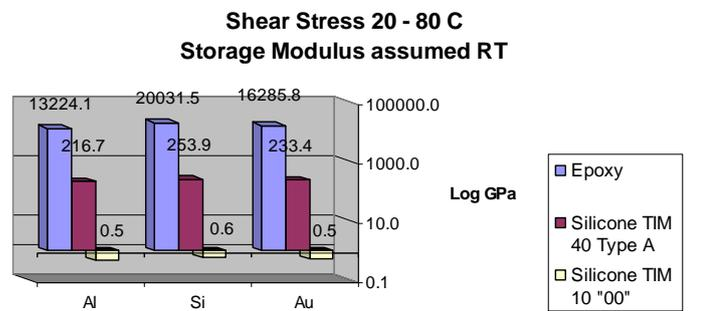
**Figure 2. Theoretical Calculated Shear Stress**
