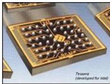
Figure 6. DSBGA packaged ICs are rarely perfectly square but they will likely be designed to furnish a uniform contact matrix for efficient second level assembly.
